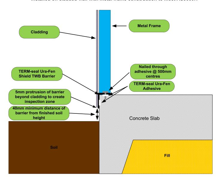
DPC is typically installed under metal frame to prevent corrosion. TERM-seal Ura-Fen Shield TWB is approved for use as a DPC so we can install under frame and bond to vertical edge of slab.
